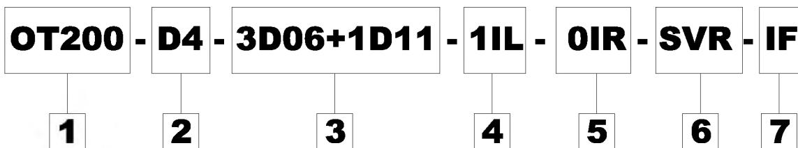
The above table example of ordering code is for a 4 elements flow divider with three 6 cc/rev element, with one intermediate lateral inlet section and another front left side inlet section.
